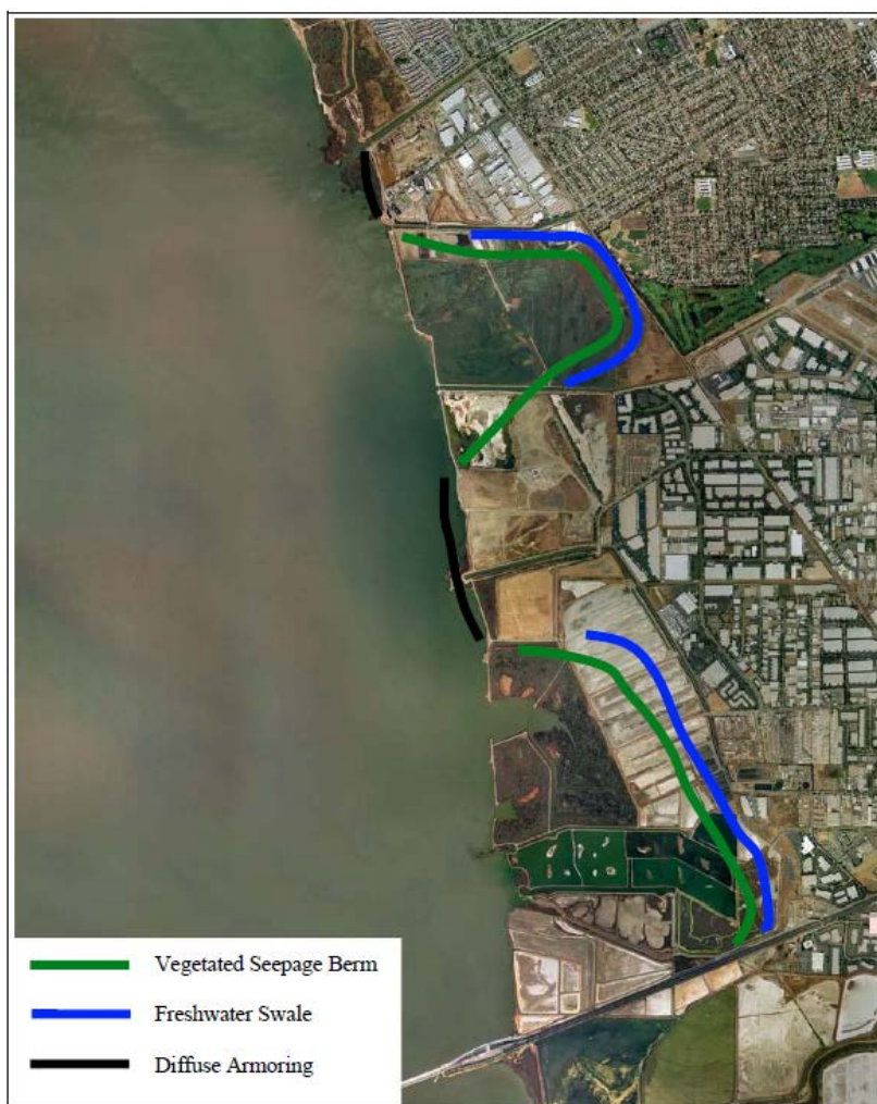
Figure 26. Design elements for a flood protection levee with upland-wetland ecotone.
